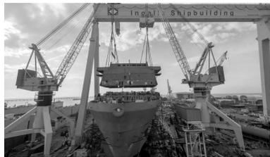
Ingalls shipbuilders set a new shipyard record Dec. 6 with the lift of the deckhouse on *John P. Murtha* (LPD 26).
